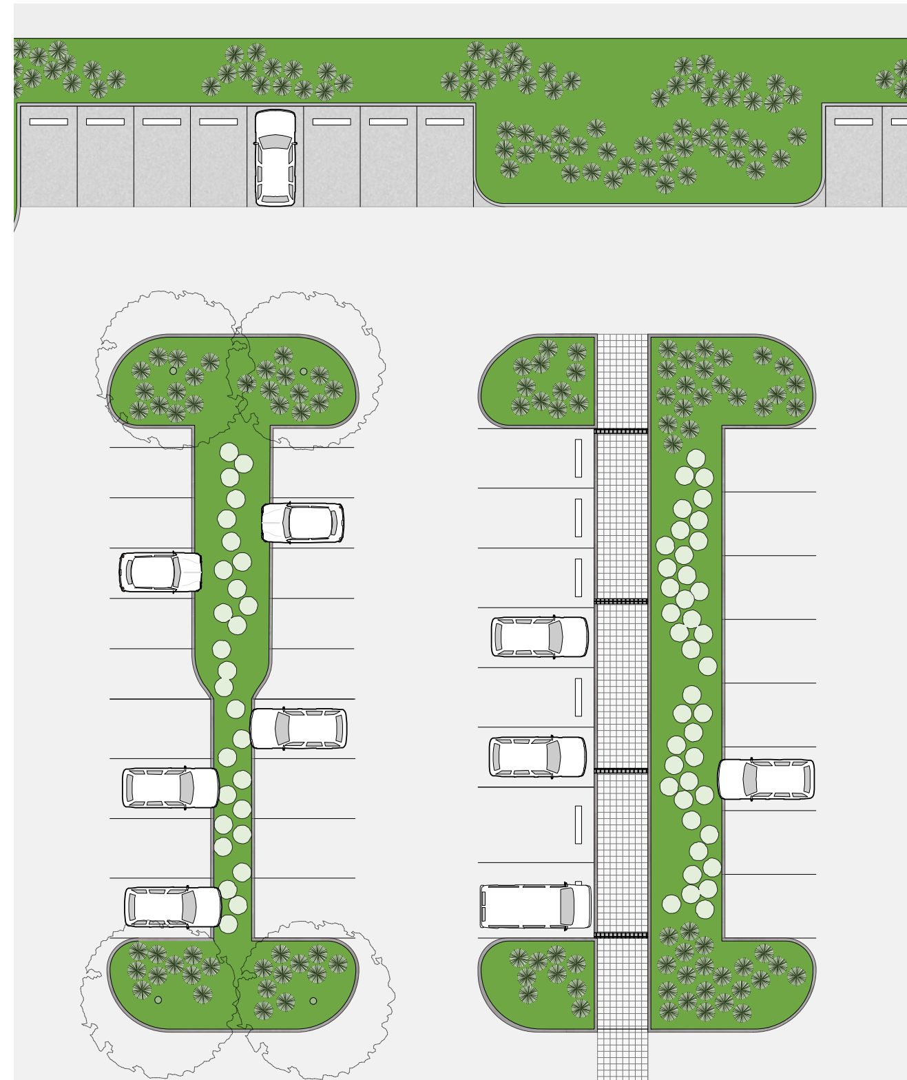
Continuous cross slope conveys the full aisle to an adjacent swale.
