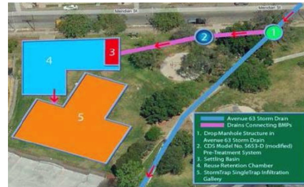
Construction of the below-ground water treatment facility at Garvanza Park in Los Angeles (left); Project features such as storm drains, sedimentation, retention and settling basins, pre-treatment systems and infiltration gallery (right)
