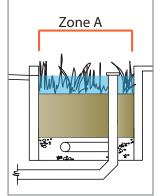
**Uniform surface grade:** This stormwater planter has a flat bottom with consistent depth of ponding across the structure. All of the plants selected for this design must be tolerant of periodic inundation (Zone A).
