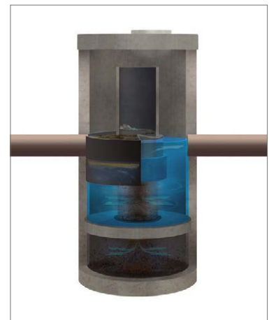
Hydrodynamic separator removes pollutants
