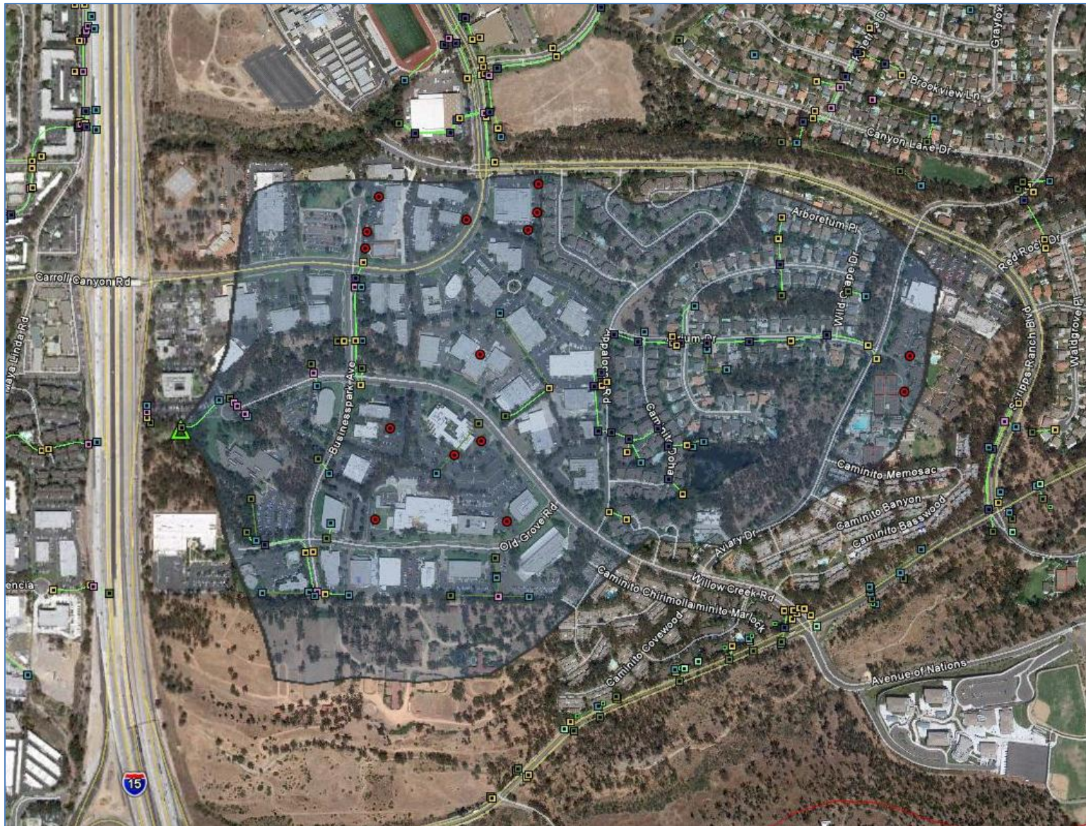
Figure B-7. Map of MS4-LPC-02 Monitoring Station and Drainage Area, including storm drain network and pollutant sources (red).
