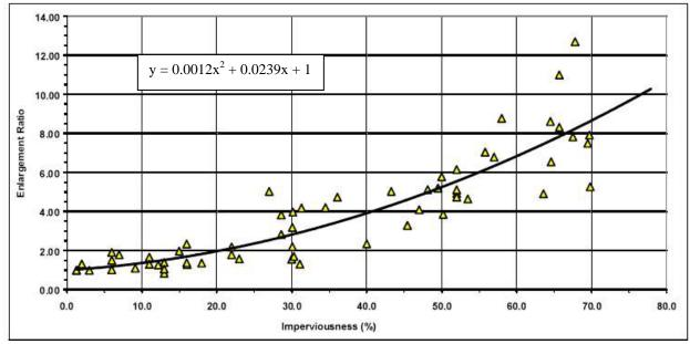
Figure 8.1 Channel Enlargement Ratio Versus Impervious Cover
