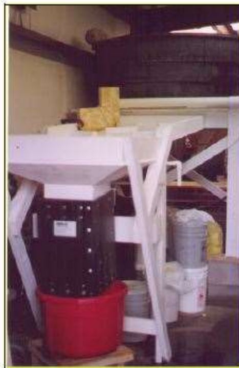
Figure 1. Flume with Ultra Urban Filter - CO in place.
