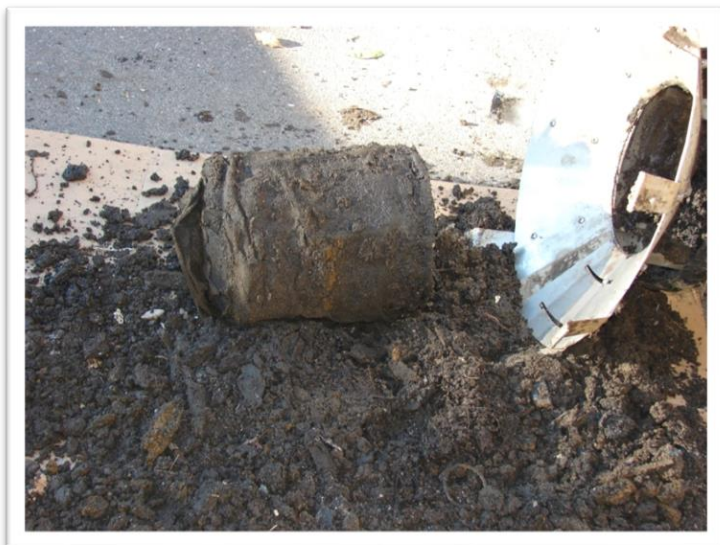
Image 5: Decomposed leaves after the Fall season and leaf drop. This area was not properly street swept and all the leaves went down the catch basin and into the unit.
