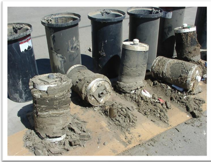
Image 4: Sediment accumulation on units after one year.
