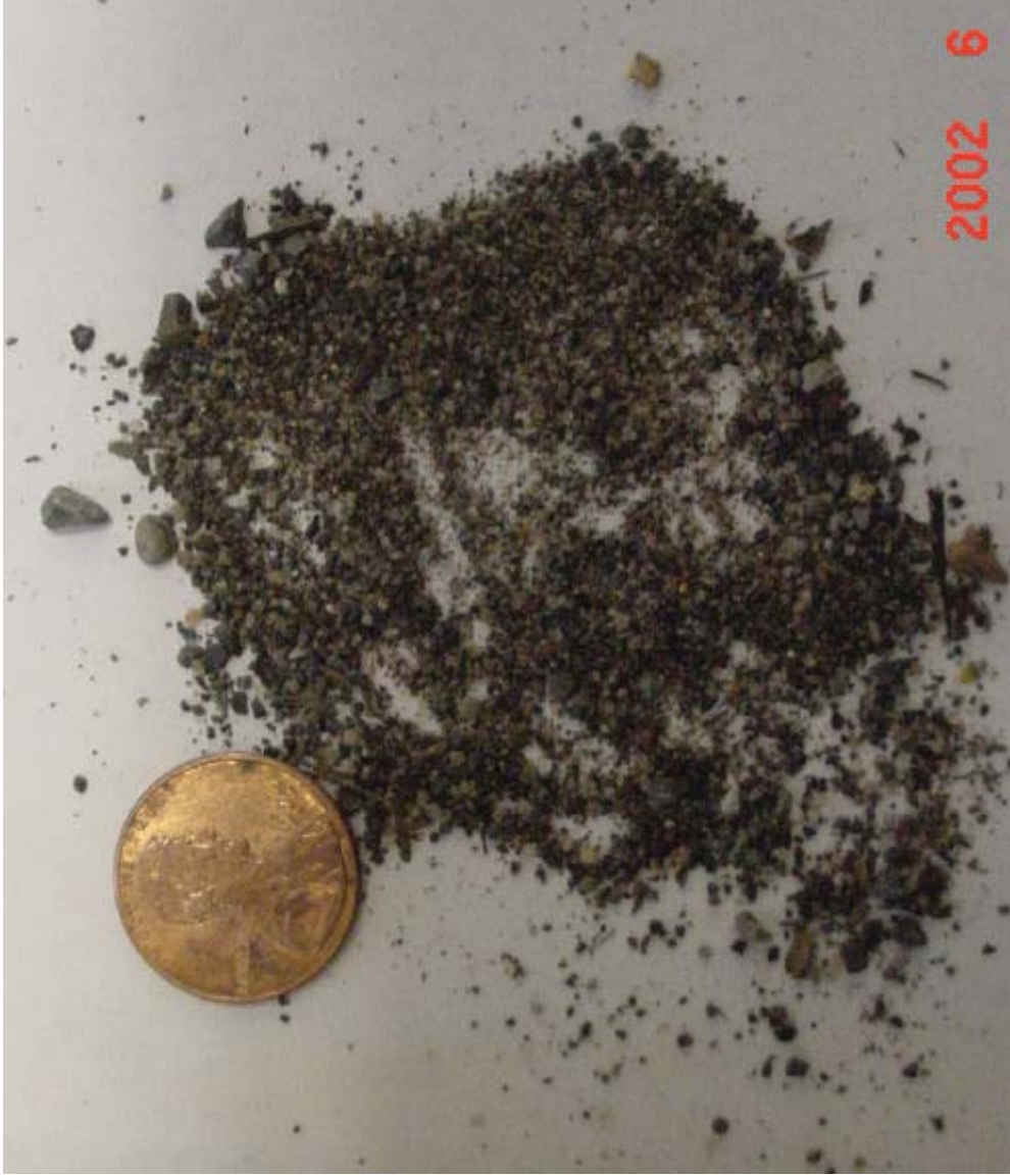
Influent Stormwater Vortex Unit Solids Sample: Coarse to Medium Grit
