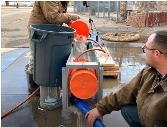
Image 3 - Introduction of trash into CFS-TD test platform with ~153GPM of water flow
