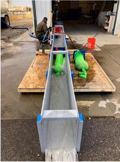
Image 9 - View looking upstream with CFS-TD and MB in trench drain test platform and small orifice screen at outlet to capture any trash that might escape (which none did)
