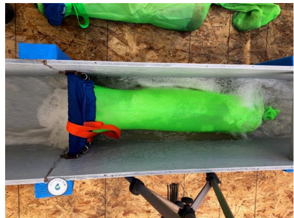
Image 8 - 153 GPM water flow with 100% trash capture in MB
