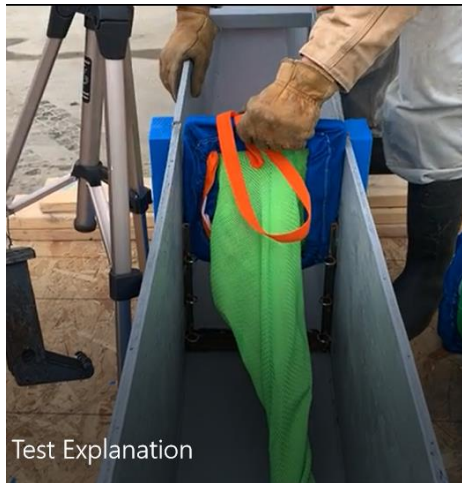
Image 7 - Mundus Bag™ partially removed from CFS-TD frame by pulling upward
