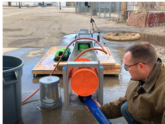
Image 4 - CFS-TD test platform with sustained water flow after trash recipe introduction
