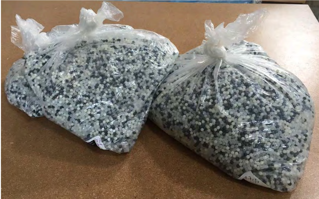
Figure 2. Plastic Spheres used to mimic gross pollutants.
