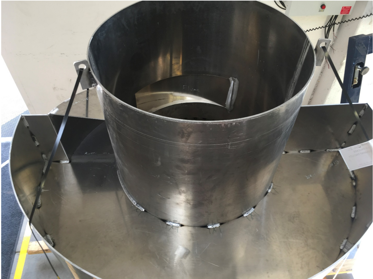
Figure 6. High Stress, High Flow Resistant Metal Inlets: Non Corrosive Stainless Steel or Marine Grade Aluminum
