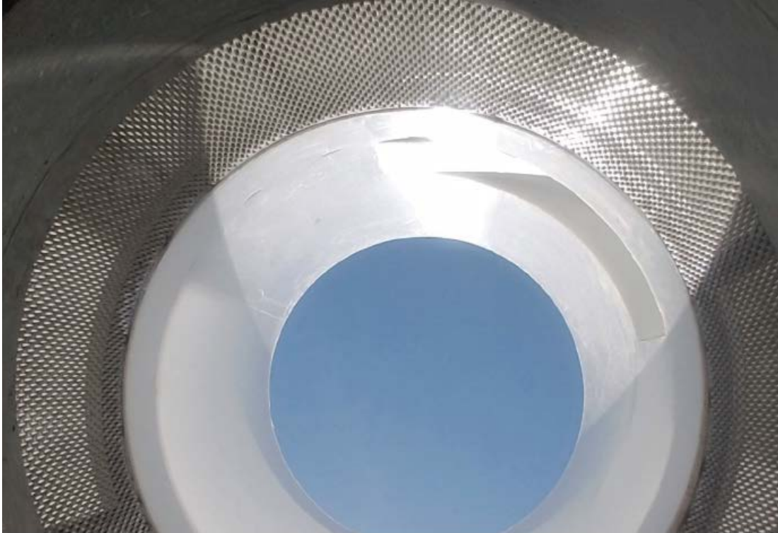
Figure 4. Bottom Up View of Separation Chamber, Showing an HDPE Inlet Riser on Top of a Stainless Steel Screen Cylinder of an Inline JDS60-2424 Unit.
