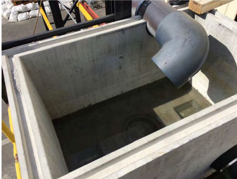
Figure 7. The D/S Sampling Chamber and free outfall for sampling.
