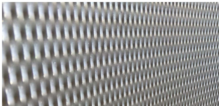
Figure 3. View of the “Blind” Side of 2,400-micron ( \mu\text{m} ), (2.4-mm) Screen Cylinder.
