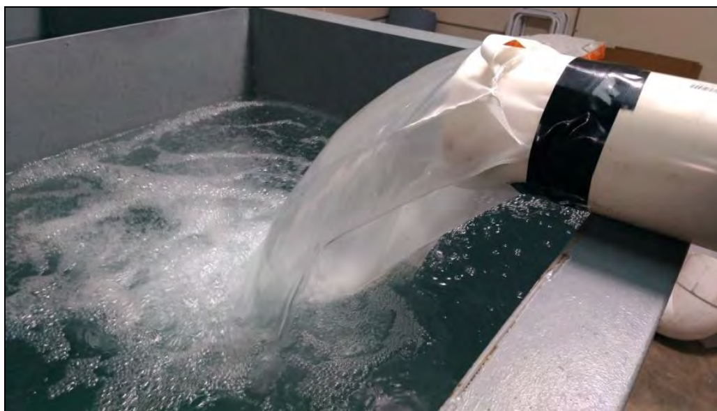
Figure 4. Net at effluent pipe discharge.
