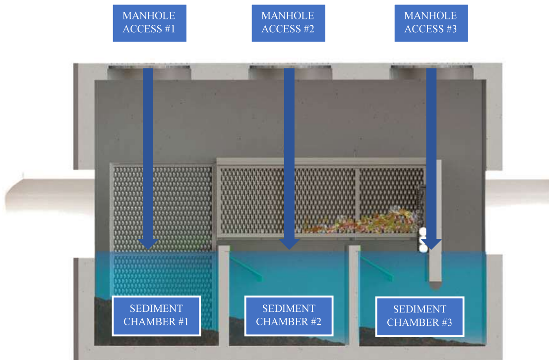
Figure 15 - Cross Section View of DSBB Showing Sediment Chambers in Relation to Access
