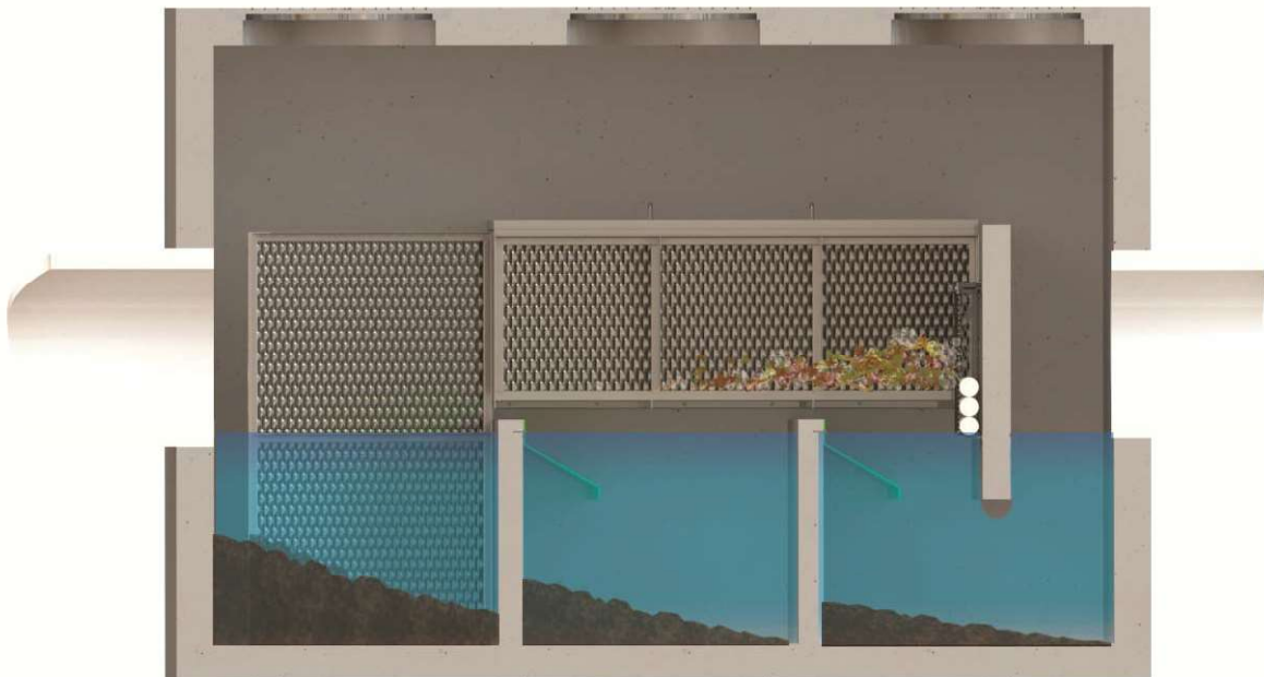
Figure 5 – DSBB Operation Between Storm Events
