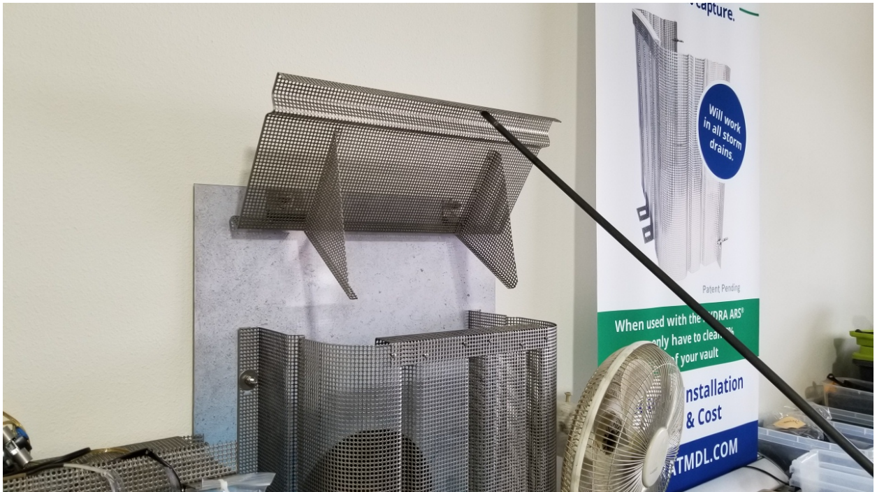
Figure 9 – CPS Bypass Lid in Open Position (bypass lid may only be open during unit maintenance or vector control access)
