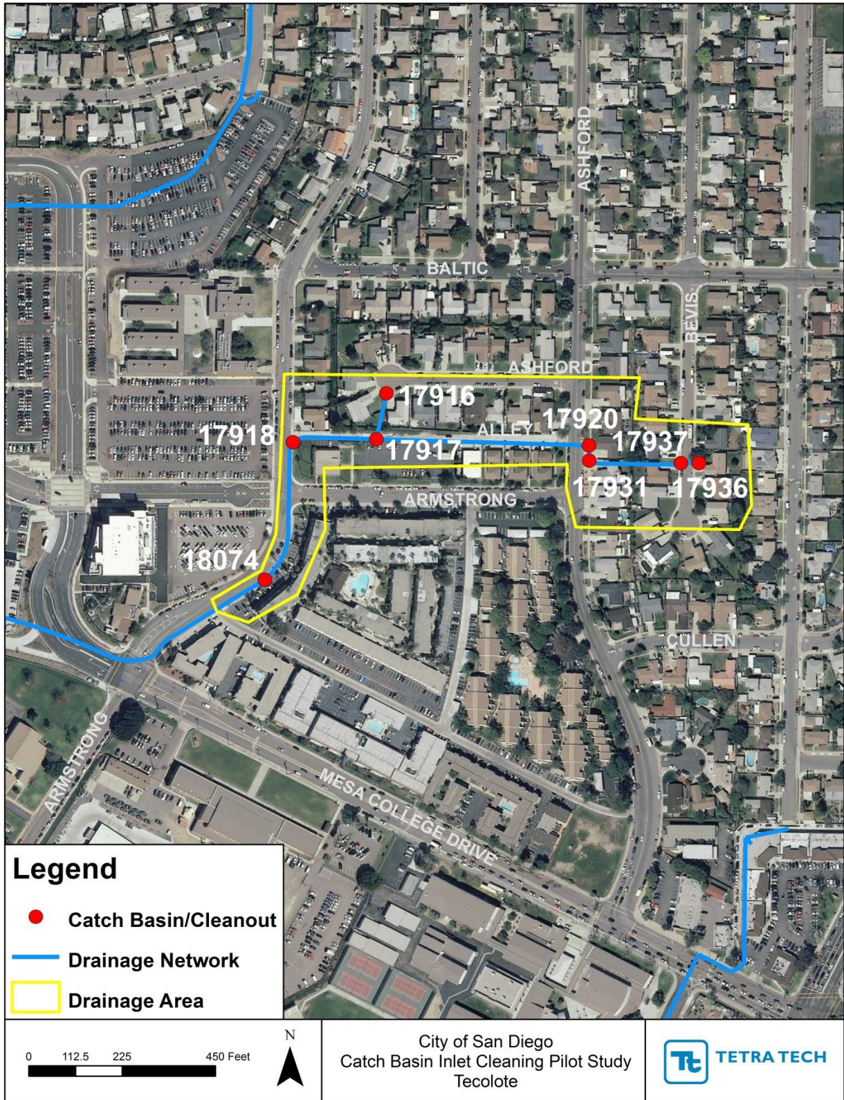
Figure 3. Tecolote drainage area and associated catch basins.
