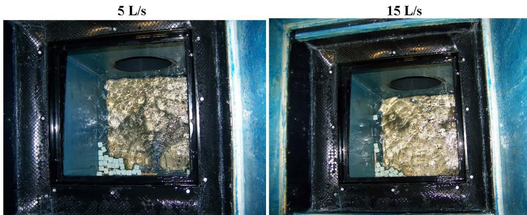
Figure 13: Retained Solids – Control at 5 and 15 L/S
