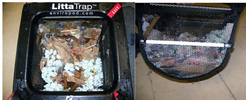
Figure 11: Retained Solids – LittaTrap™ at 15 L/s
