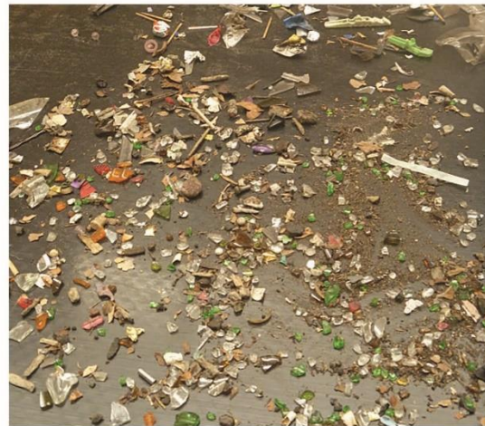
Figure 5: Other gross pollutants captured by LittaTrap
