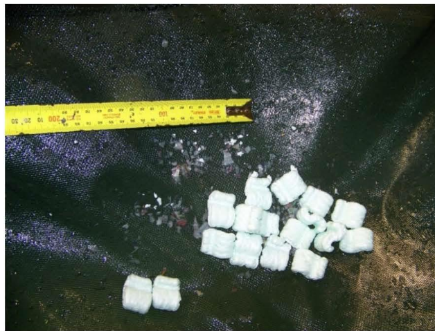
Figure 10: Escaped Solids – LittaTrap™ at 15 L/s
