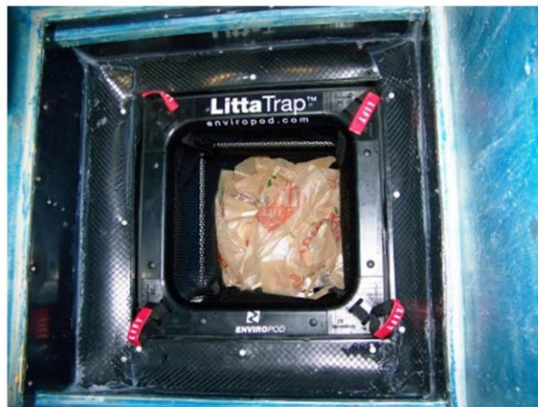
Figure 5: LittaTrap™ Scour Test Preload
