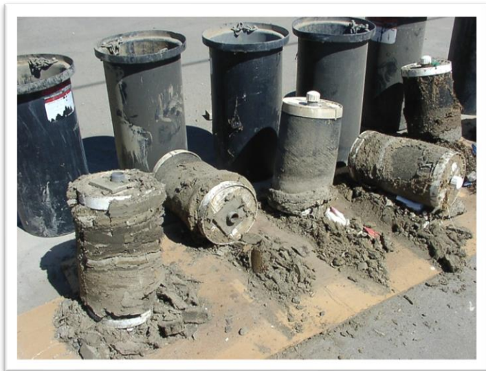
Image 11: Sediment accumulation on first generation units after one year.
