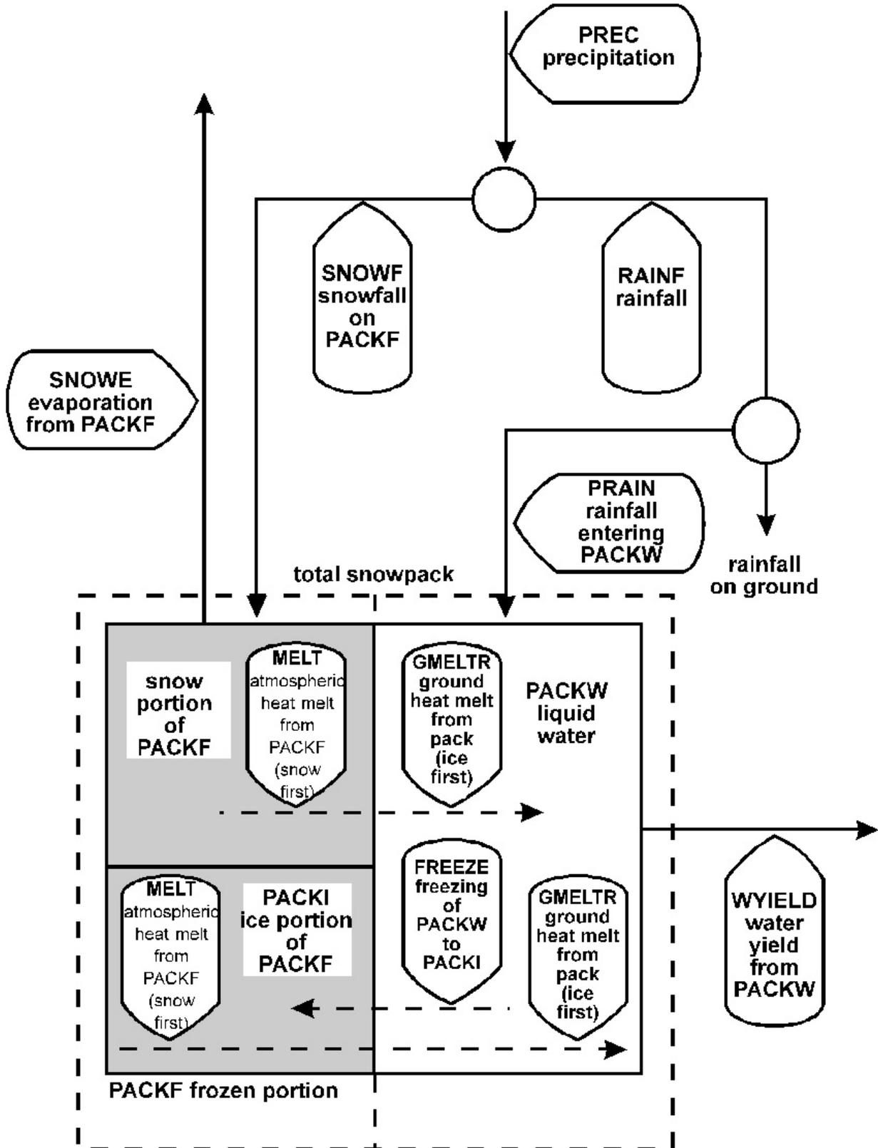
Figure 12: Flow diagram of water movement, storages, and phase changes modeled in the SNOW section of the PERLND and IMPLND Application Modules
