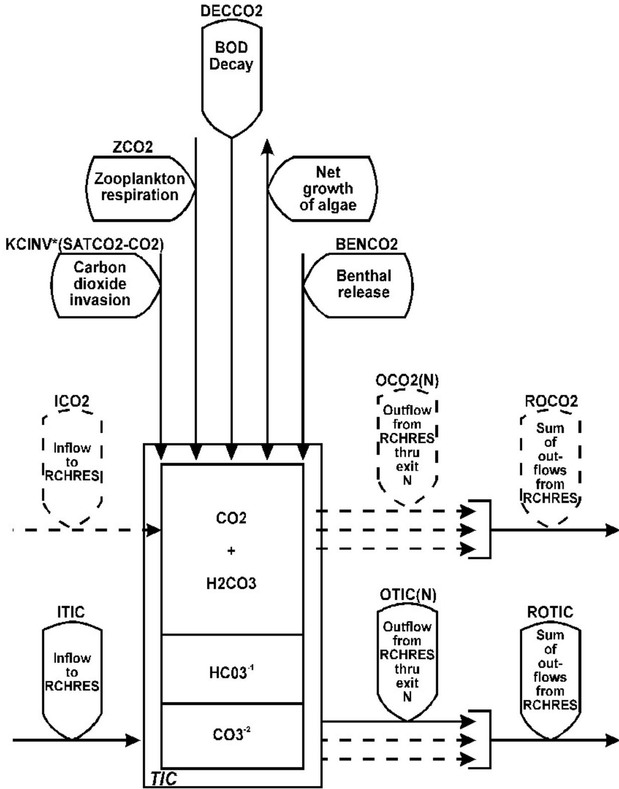
Figure 64: Flow diagram of inorganic carbon in the PHCARB group of the RCHRES Application Module
