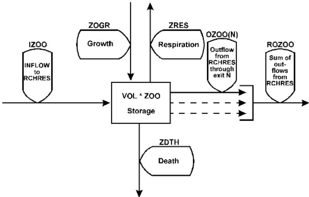
Figure 60: Flow diagram for zooplankton in the PLANK section of the RCHRES Application Module
