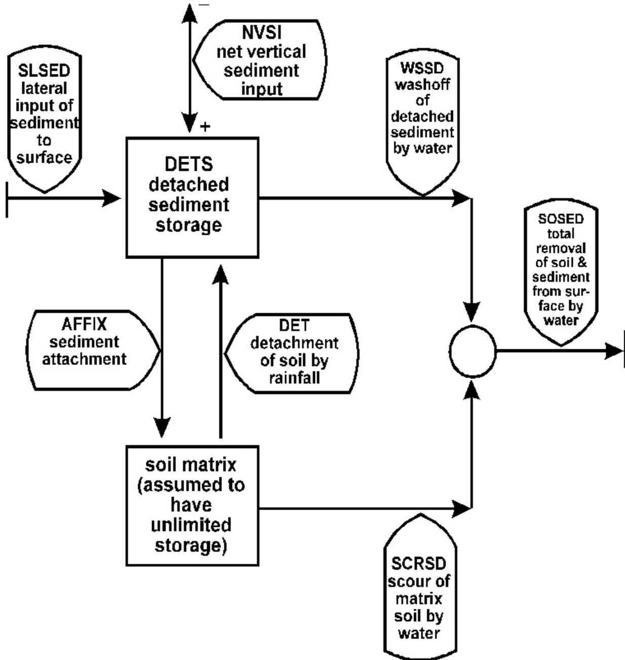
Figure 23: Flow diagram for SEDMNT section of PERLND Application Module
