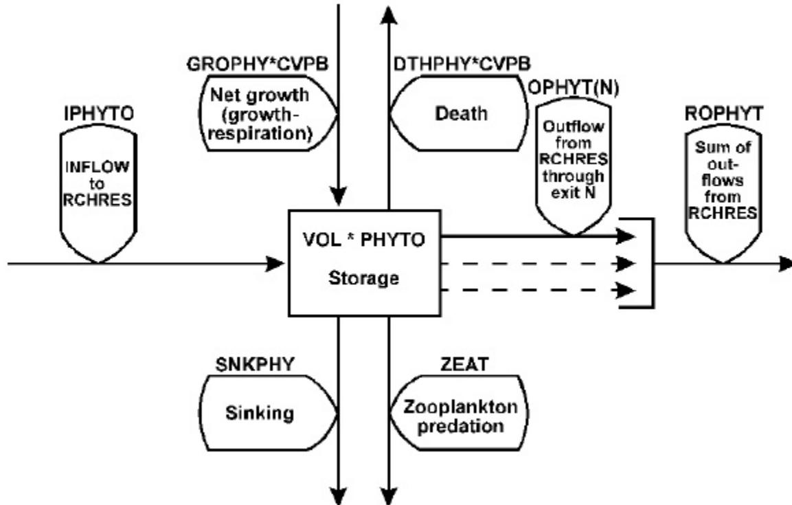
Figure 58: Flow diagram for phytoplankton in the PLANK section of the RCHRES Application Module
