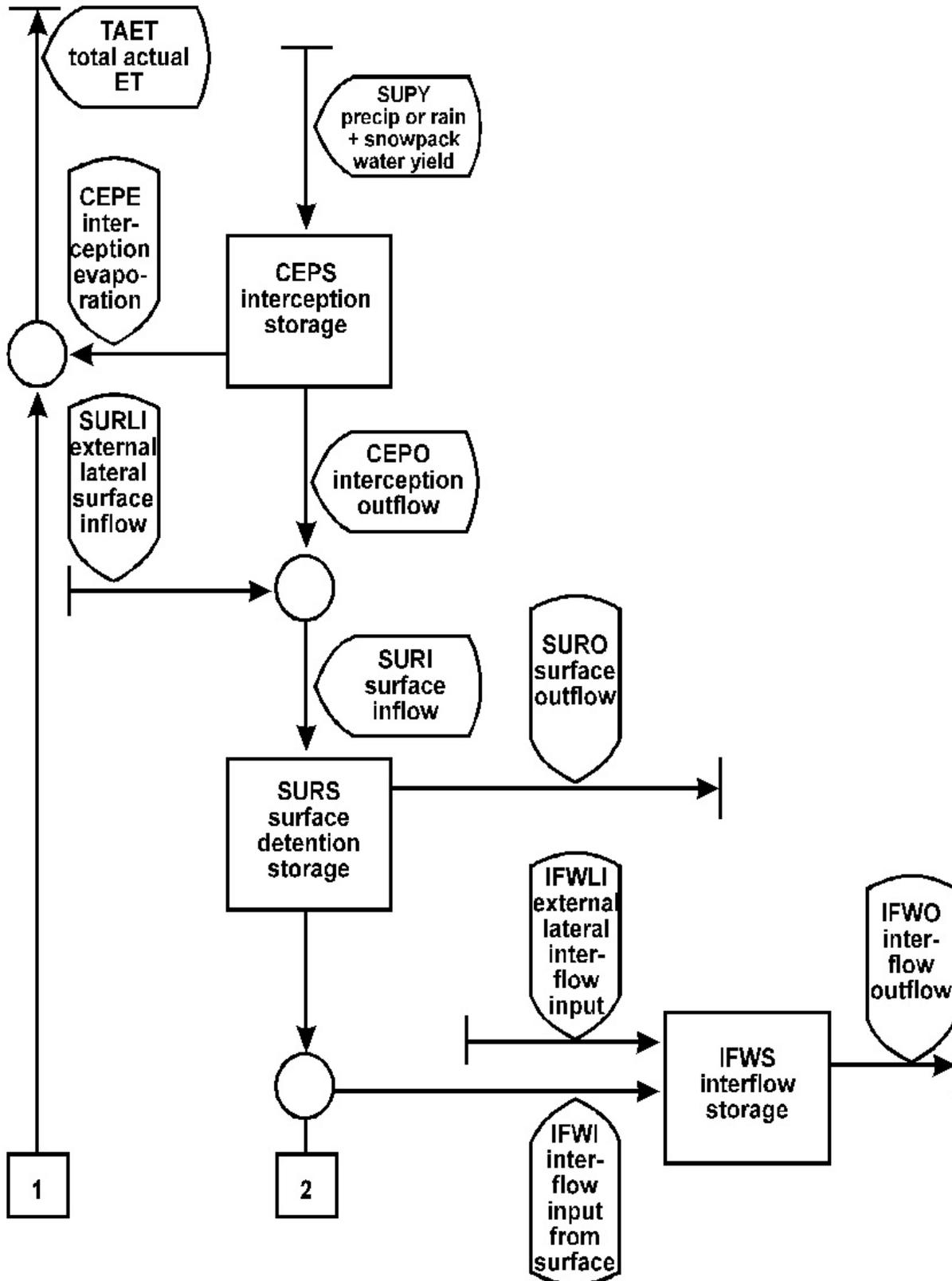
Figure 14: Flow diagram of water movement and storages modeled in the PWATER section of the PERLND Application Module
