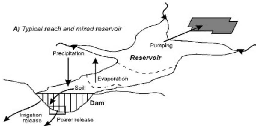
Figure 39: Typical RCHRES configurations and the method used to represent geometric and hydraulic properties
