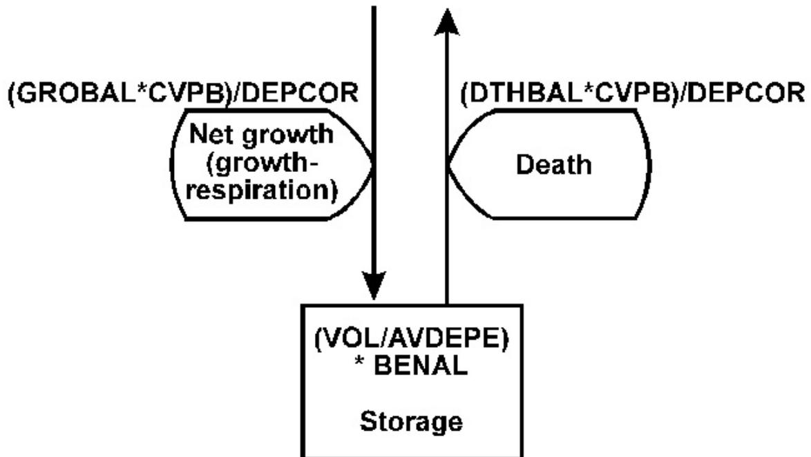
Figure 61: Flow diagram for benthic algae in the PLANK section of the RCHRES Application Module
