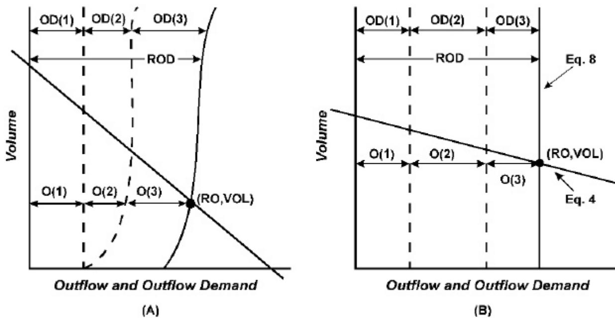
Figure 38: Graphical representation of the equations used to compute outflow rates and volume
