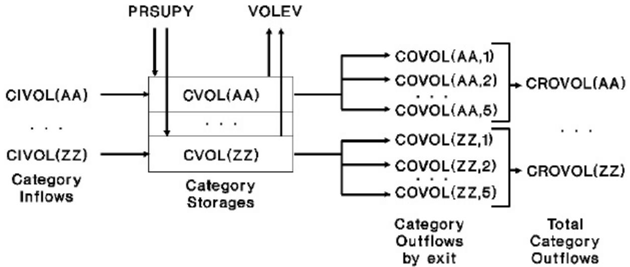
Figure 43: Flow diagram for water categories in the HYDR Section of the RCHRES Application Module
