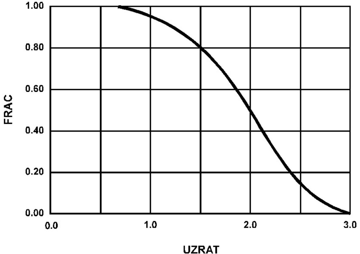
Figure 17: Fraction of the potential direct runoff retained by the upper zone (FRAC) as a function of the upper zone soil moisture ratio (UZRAT)
