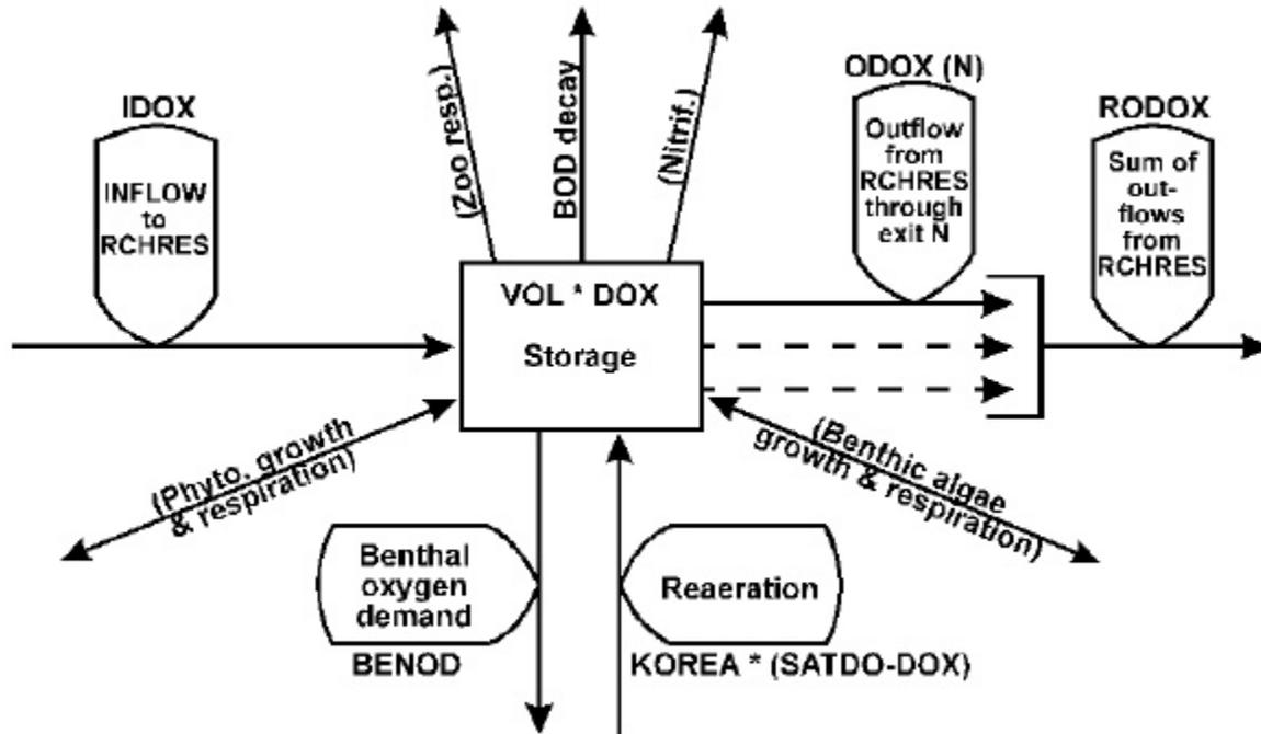
Figure 54: Flow diagram for dissolved oxygen in the OXRX subroutine group of the RCHRES Application Module
