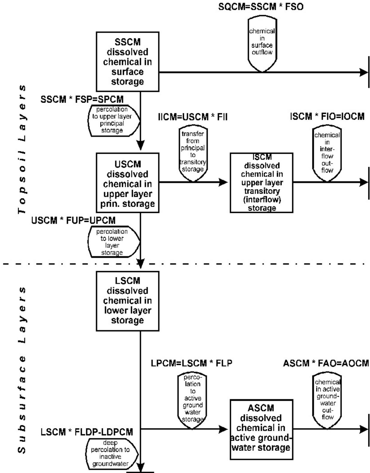
Figure 26: Flow diagram showing modeled movement of chemicals in solution
