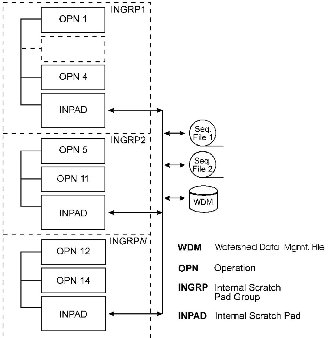
Figure 7: Schematic of data flow and storage for a single run
