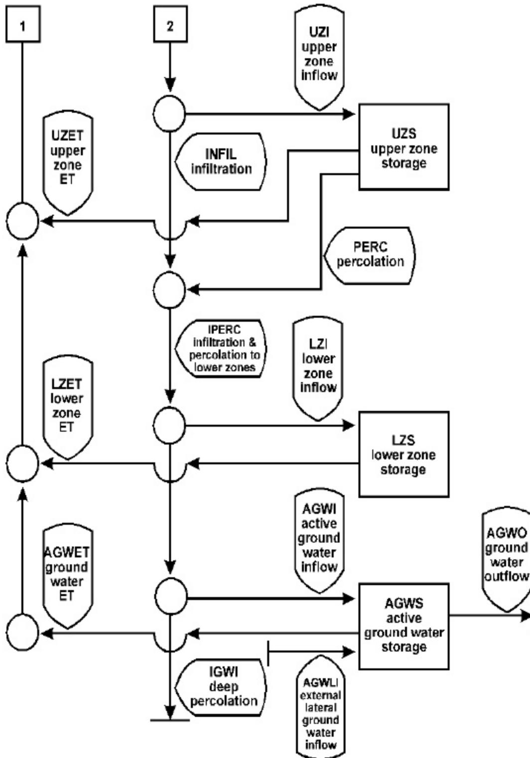
Figure 15: Flow diagram of water movement and storages modeled in the
