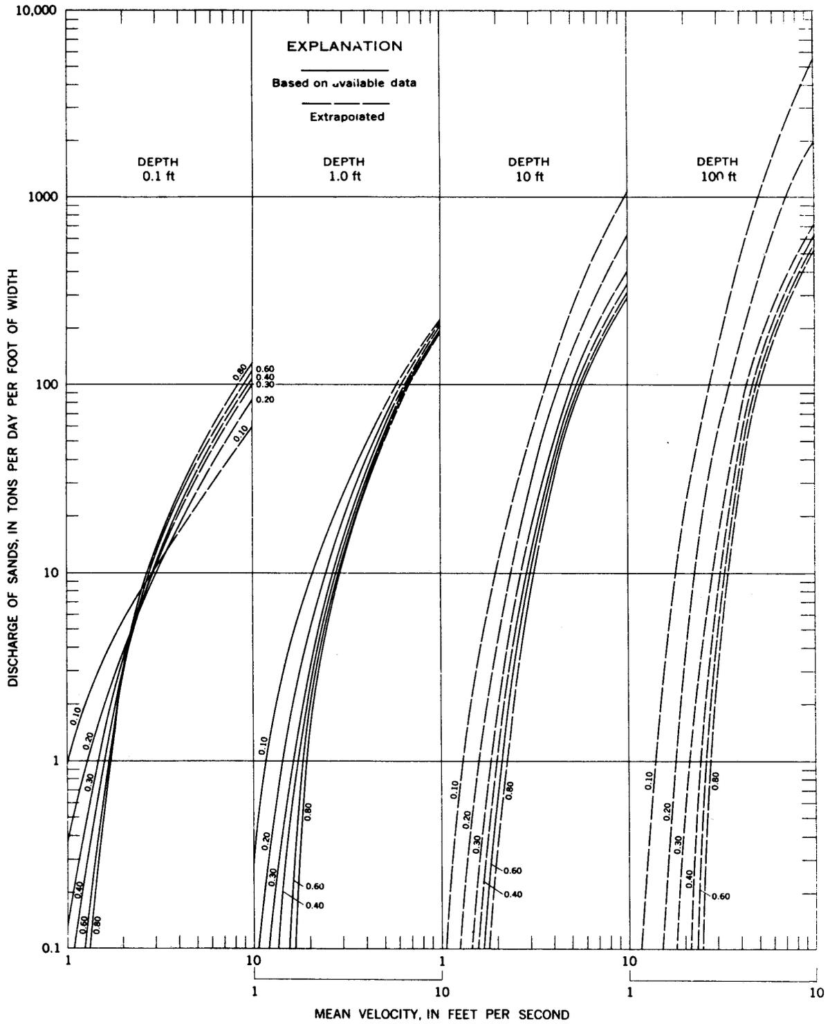
Figure 50: Colby's relationship for discharge of sands in terms of mean velocity for six median sizes of bed sands, four depths of flow, and water temperature of 60 F
