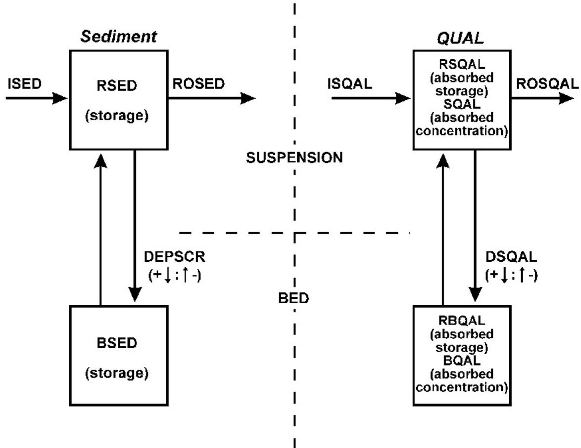
Figure 53: Simplified flow diagram for important fluxes and storages of sediment and associated qual used in subroutine ADVQAL
