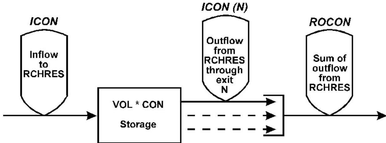
Figure 45: Flow diagram for conservative constituents in the CONS section of the RCHRES Application Module
