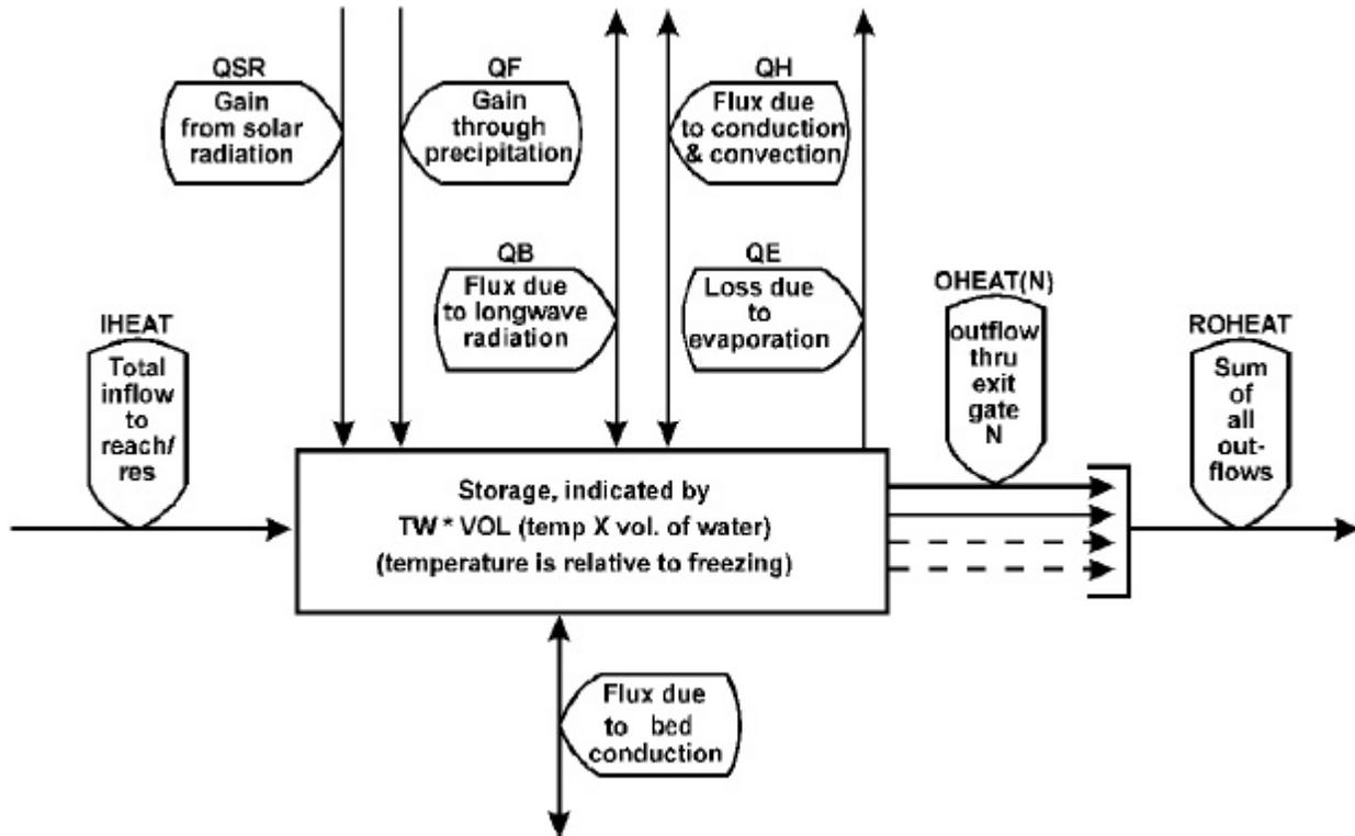
Figure 46: Flow diagram for HTRCH section of the RCHRES Application Module
