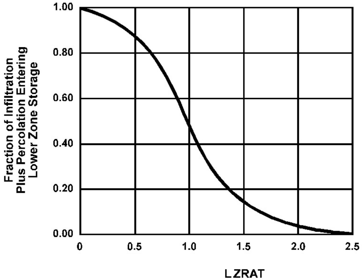
Figure 18: Fraction of infiltration plus percolation entering lower zone storage
