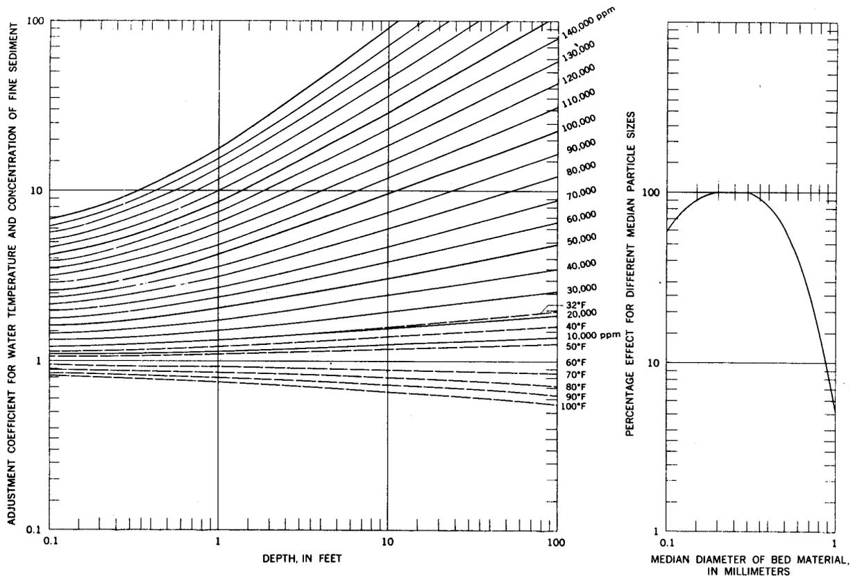
**Figure 51: Colby's correction factors for effect of water temperature, concentration of fine sediment, and sediment size; applied to uncorrected discharge of sand given by above graph**
