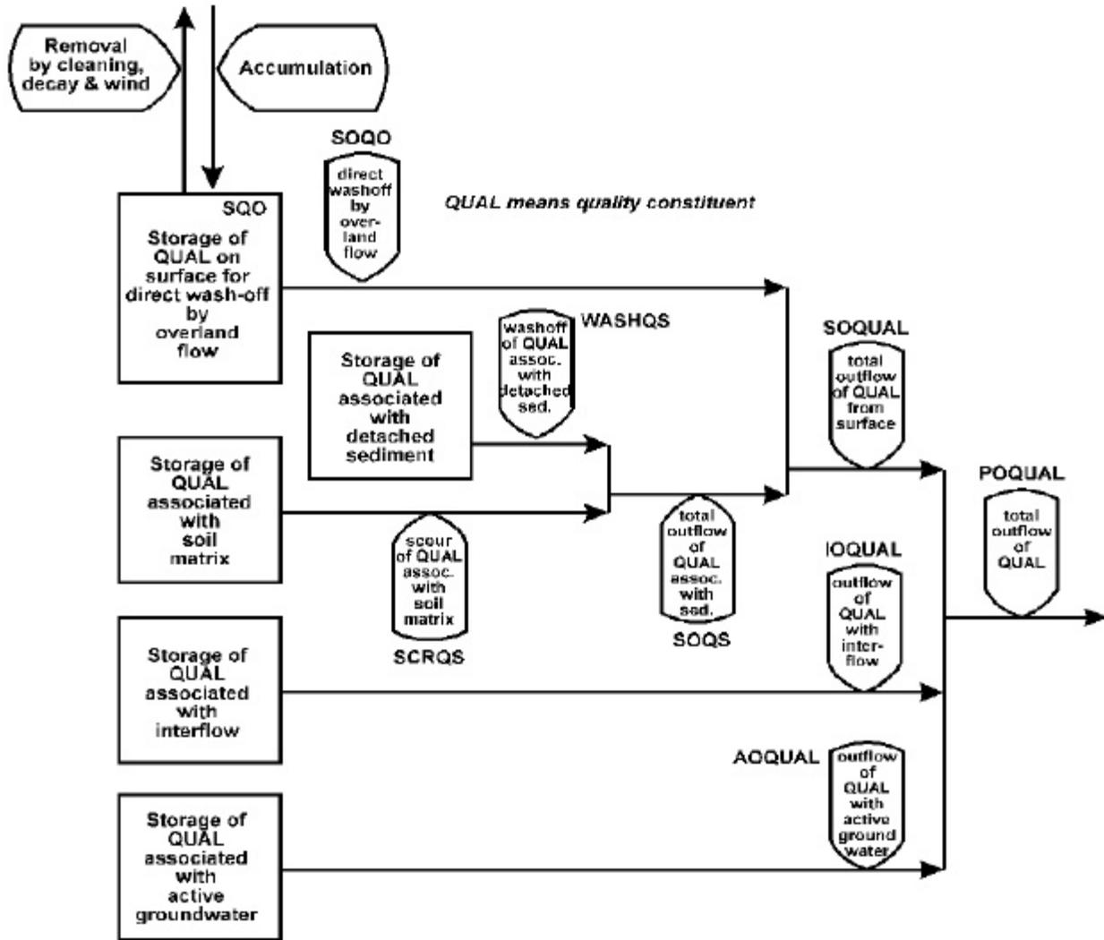
Figure 24: Flow diagram for PQUAL section of the PERLND Application Module
