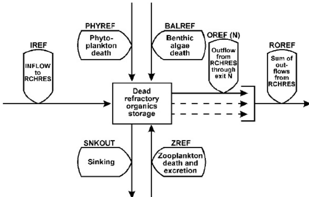
Figure 59: Flow diagram for dead refractory organics in the PLANK section of the RCHRES Application Module
