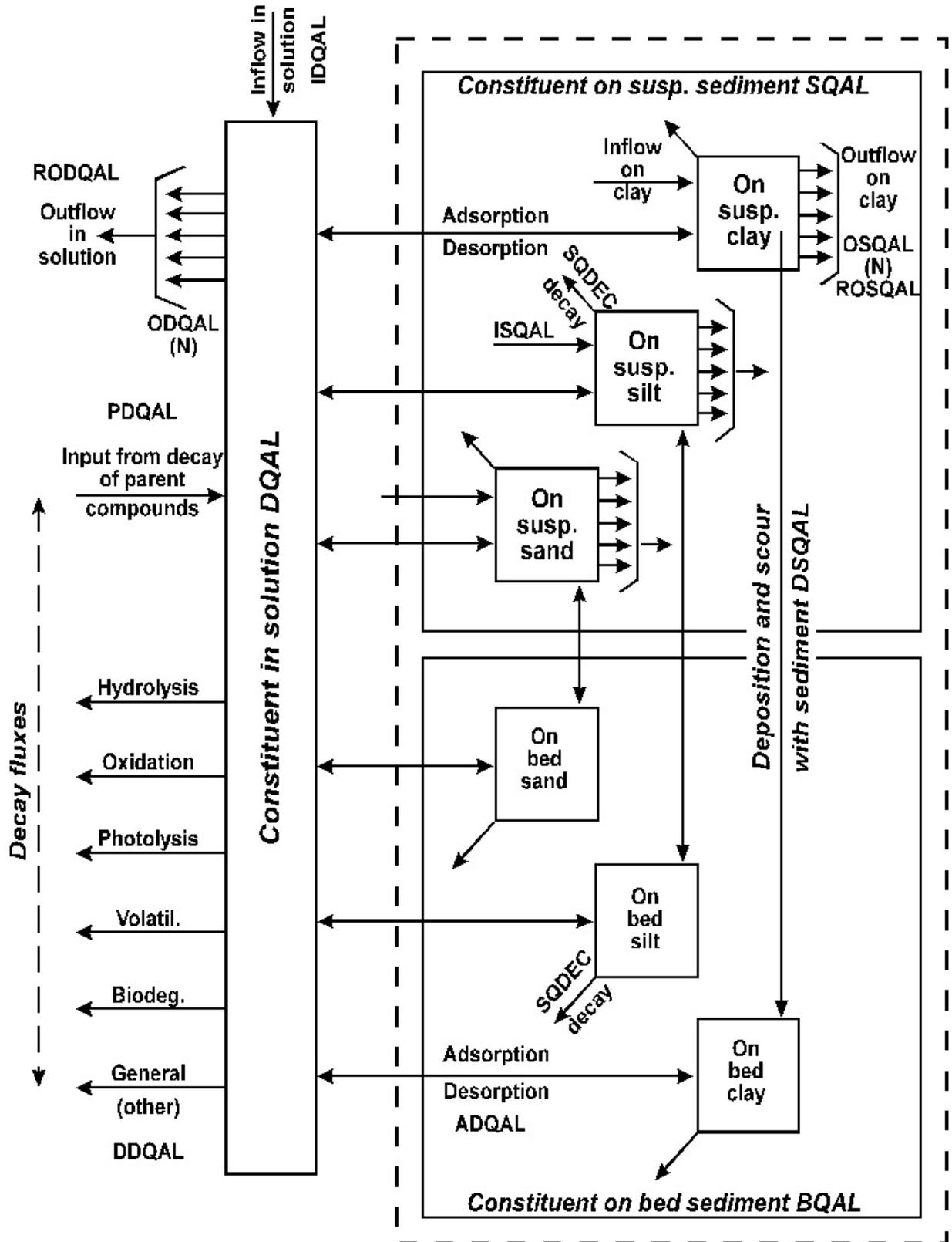
Figure 52: Flow diagram for generalized quality constituent in the GQUAL section of the RCHRES Application Module
