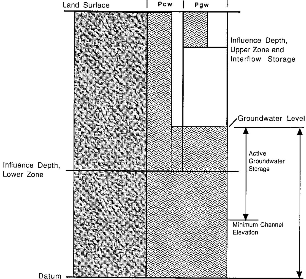
Figure 20: Sketch of soil moisture in the unsaturated zone under high water table conditions
