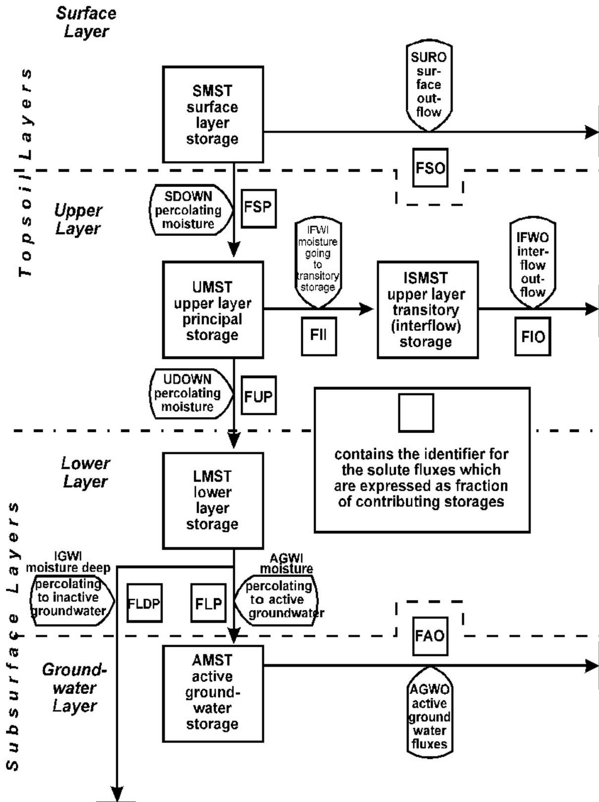
Figure 25: Flow diagram showing transport of moisture and solutes as estimated in the MSTLAY section of the PERLND Application Module
