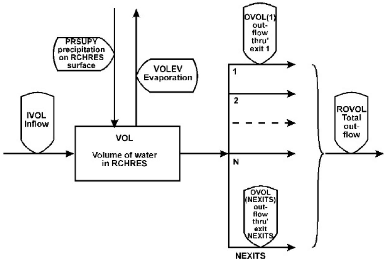
Figure 37: Flow diagram for the HYDR Section of the RCHRES Application Module
