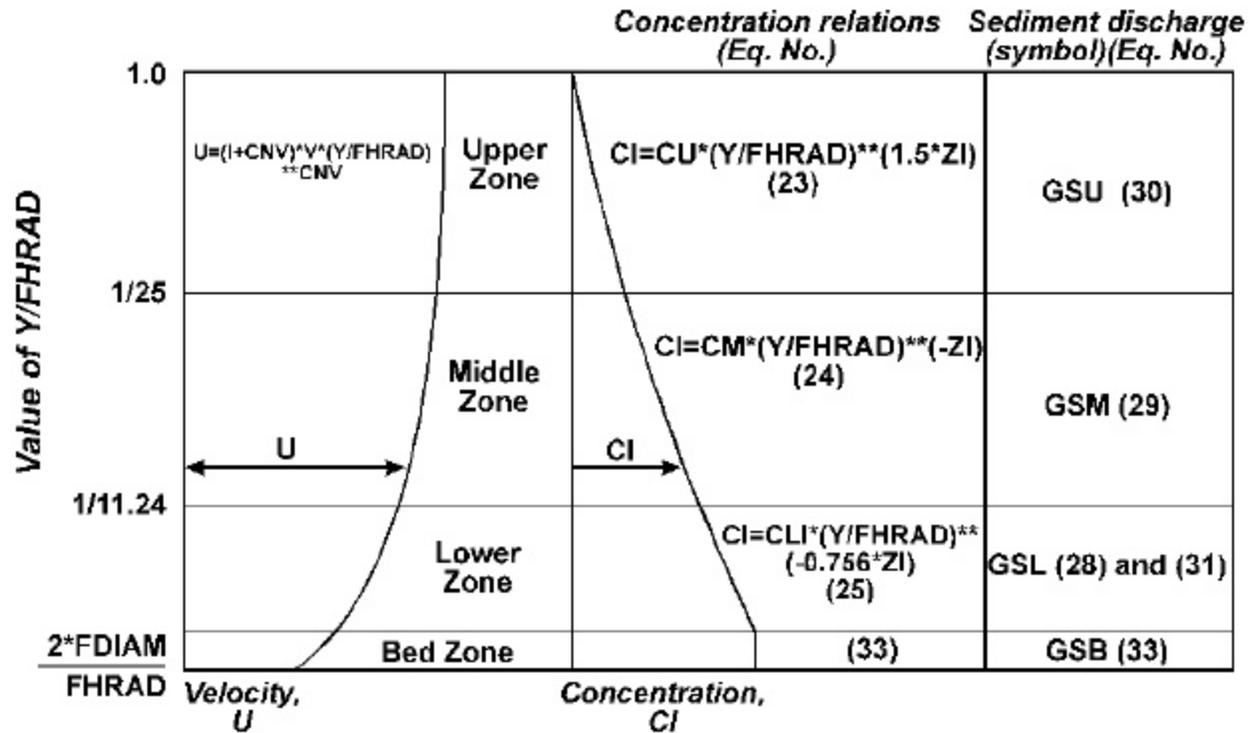
Figure 48: Toffaleti's velocity, concentration, and sediment discharge relations
