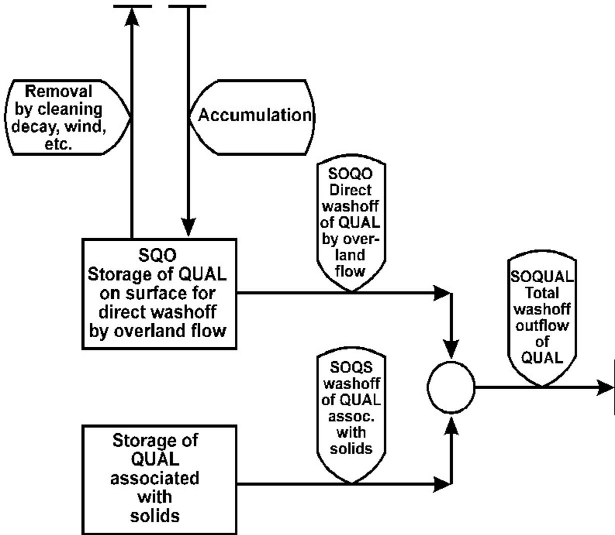
Figure 34: Flow diagram for IQUAL section of IMPLND Application Module
