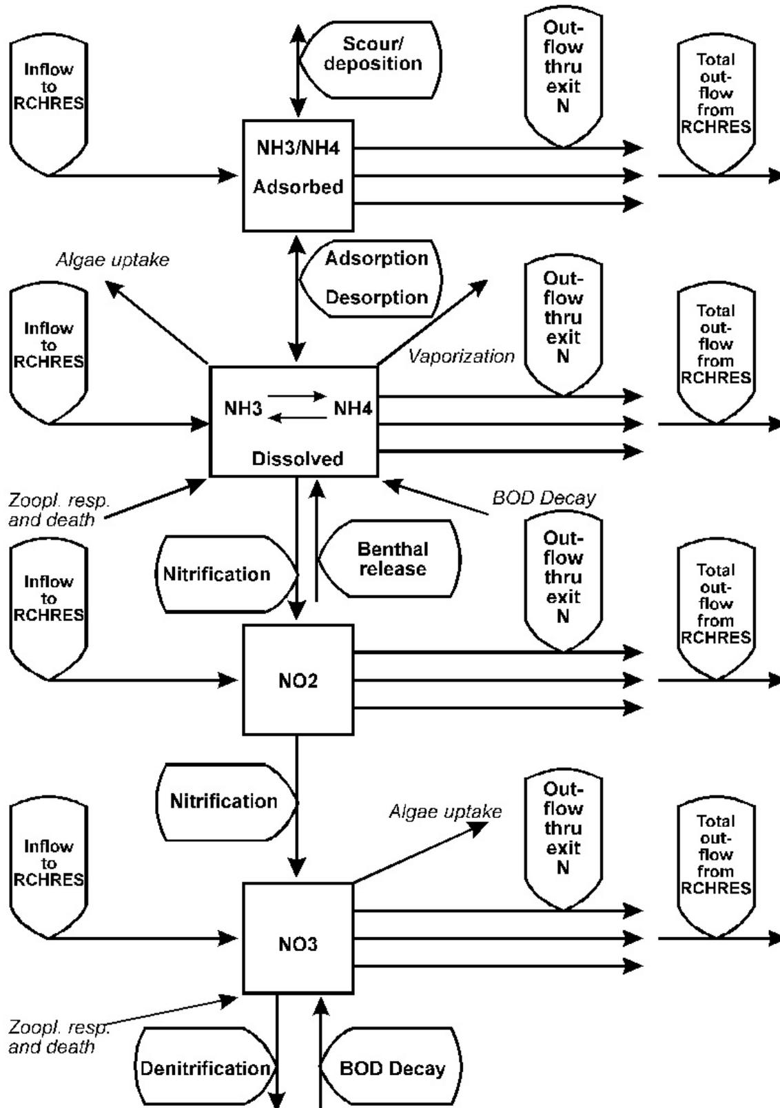
Figure 56: Flow diagram for inorganic nitrogen in the NUTRX subroutine group of the RCHRES Application Module
