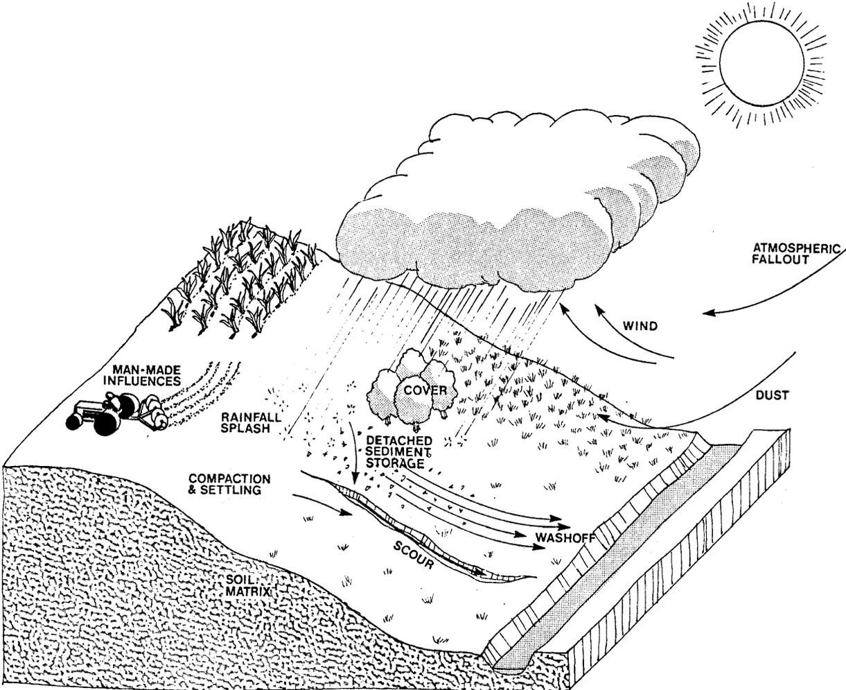
Figure 22: Erosion processes
