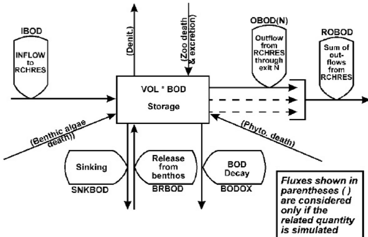
Figure 55: Flow diagram for biochemical oxygen demand in the OXRX subroutine group of the RCHRES Application Module
