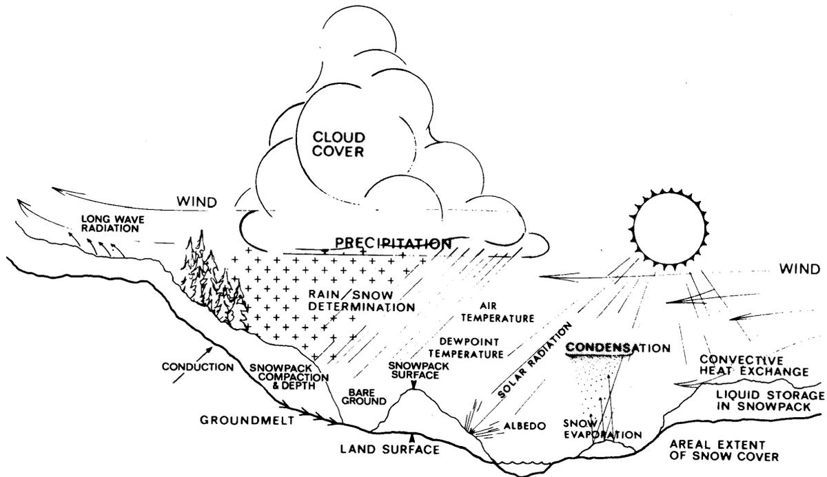
**Figure 11: Snow accumulation and melt processes**
