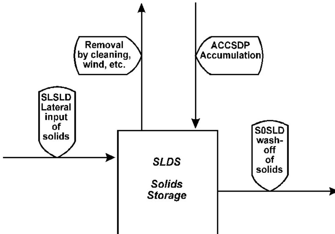
Figure 33: Flow diagram of the SOLIDS section of the IMPLND Application Module
