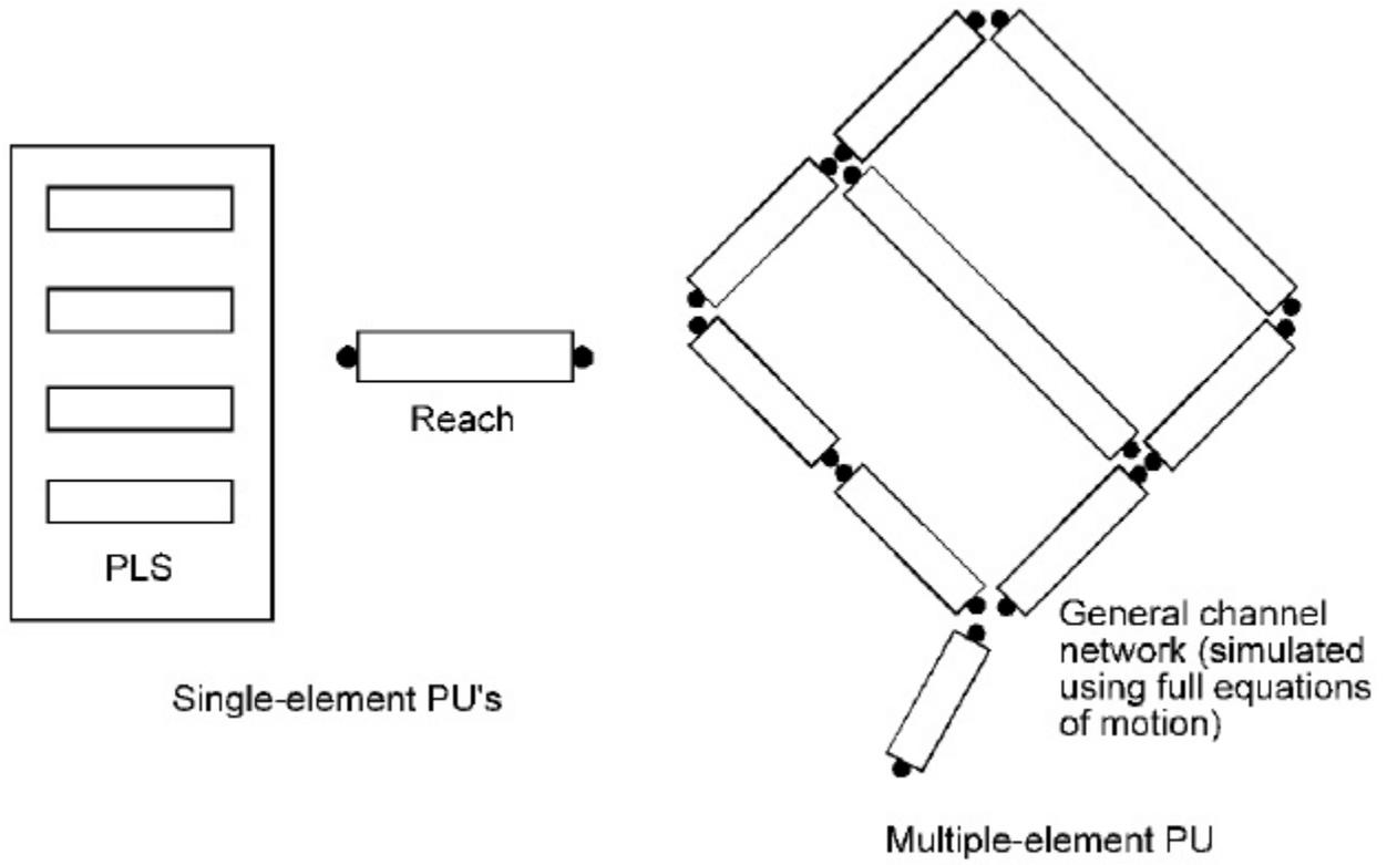
Figure 3: Single- and multi-element processing units
