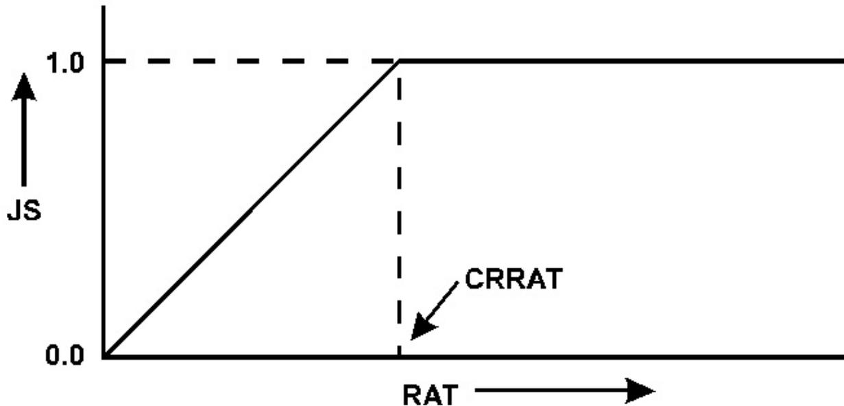
Figure 44: Determination of weighting factors for advection calculations
