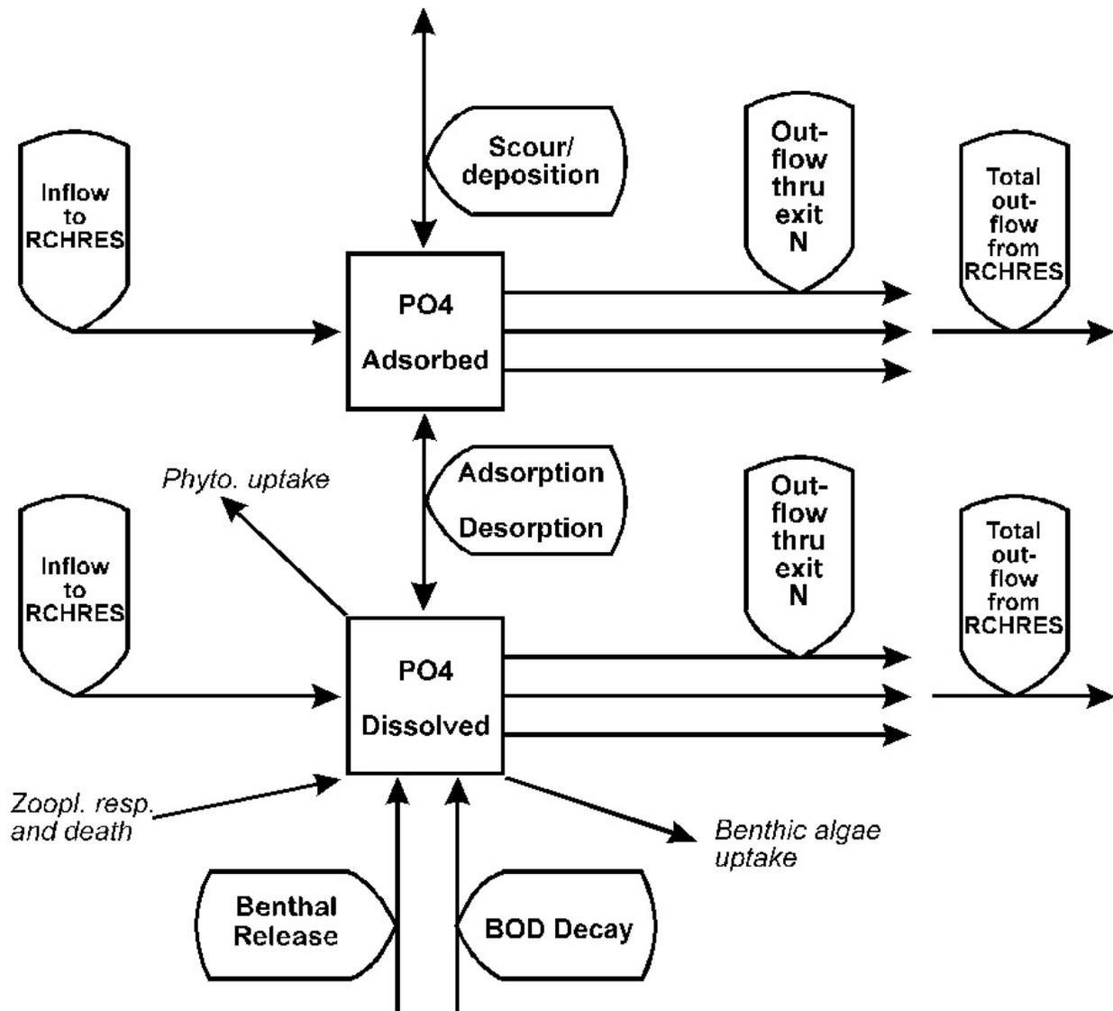
Figure 57: Flow diagram for ortho-phosphate in the NUTRX subroutine group of the RCHRES Application Module
