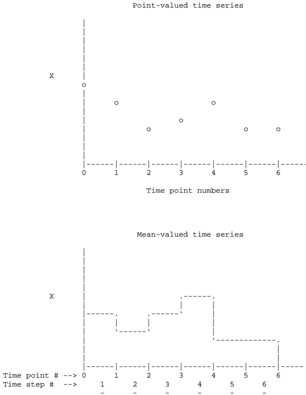
**Figure 75: Comparison between point- and mean-valued time series**
