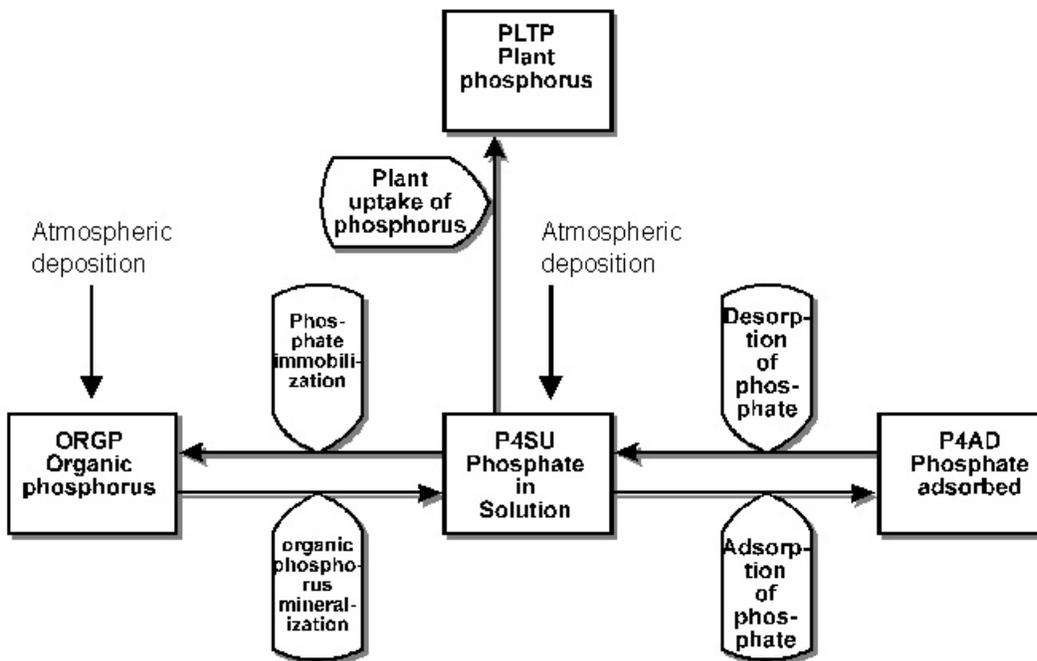
Figure 29: Flow diagram for phosphorus reactions
