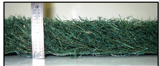
A side view of the Bioflex. (1.75" thick allows for longer filtration times due to the 3 dimensional webbing.
