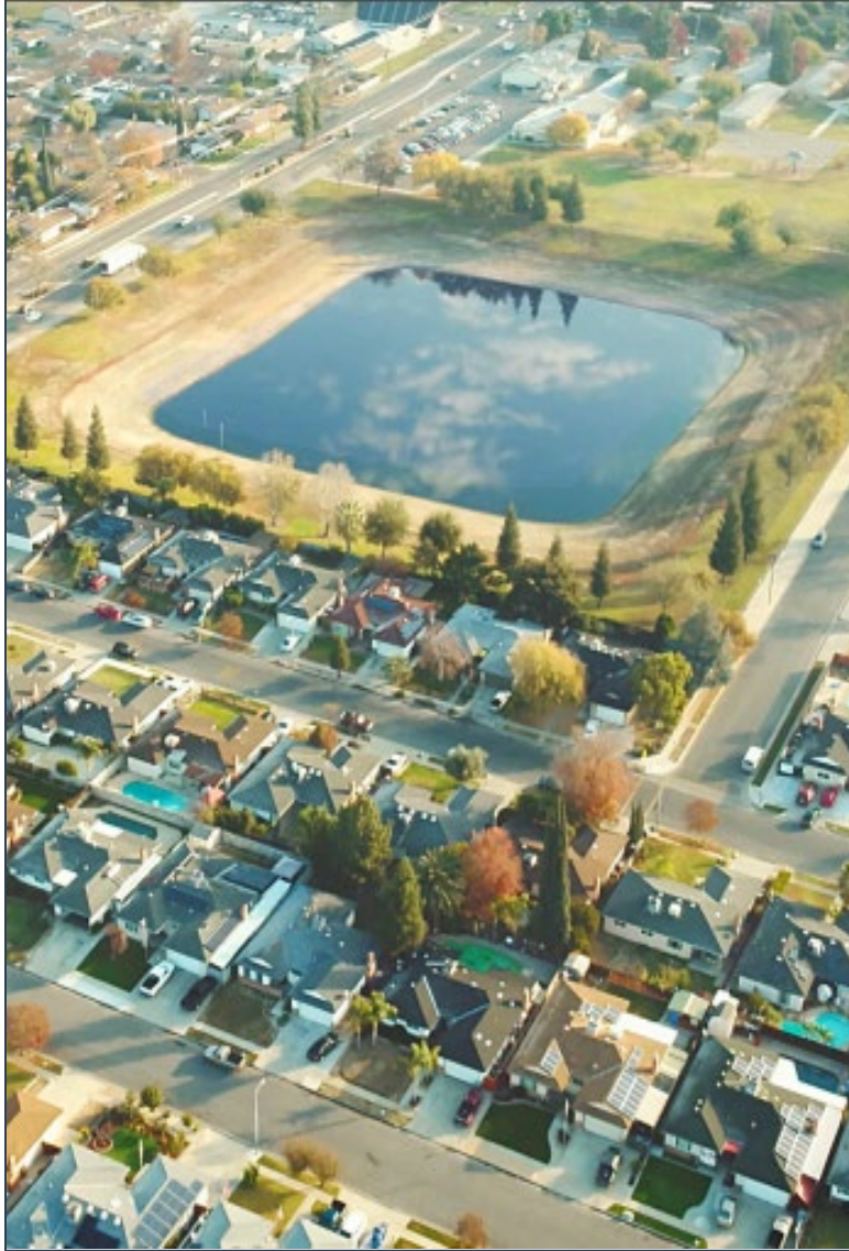
Figure 8: Example of a stormwater capture basin in the FMFCD system surrounded by limited greenspace (Fresno Metropolitan Flood Control District, 2023b).
