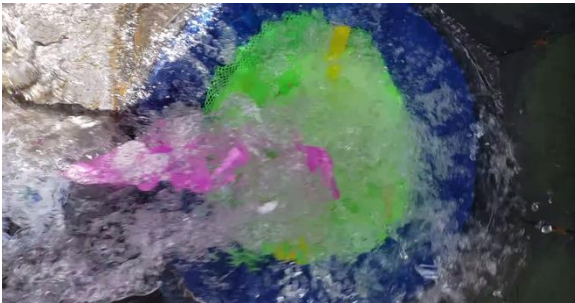
Image 22 - Overhead view of simulated trash entering TTC-MB during 500 gpm test
