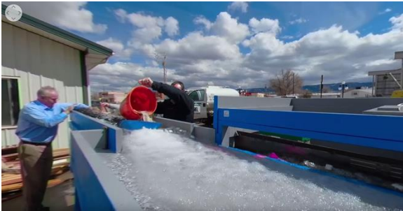
Image 20 - Introduction of simulated trash during 500 GPM test
