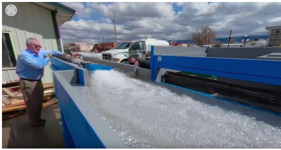
Image 18 - Test platform water introduction at 500 GPM
