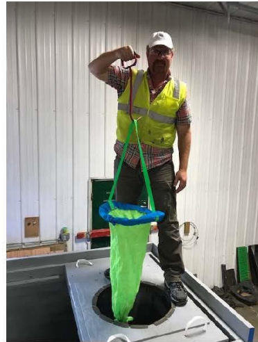
Image 6 - Mundus Bag® removal from CIF on curb inlet style catch basin test platform
