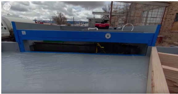
Image 16 - Test platform with curb inlet mouth and CIF visible
