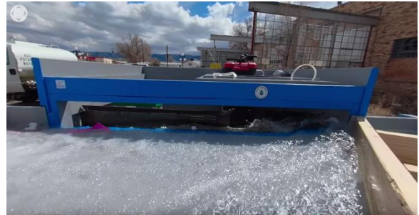
Image 21 - Simulated trash being ingested by CIF at 500 GPM
