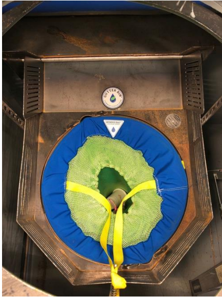
Image 13 - Fully installed CIF with interface funnel, filter hanger, and MB (TTC-MB) viewed from above
